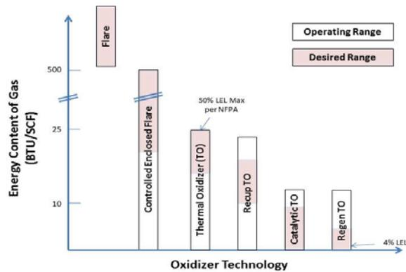
direct fired oxidizers. Processes with very low energy contribution from the combustion process are ideally treated with a regenerative thermal oxidizer or a recuperative thermal oxidizer with high heat exchanger efficiencies and potentially secondary heat recovery. Processes with low to moderate levels of energy contribution should be carefully assessed to optimize equipment efficiency versus overall energy requirements. The chart below graphically depicts this relationship:
